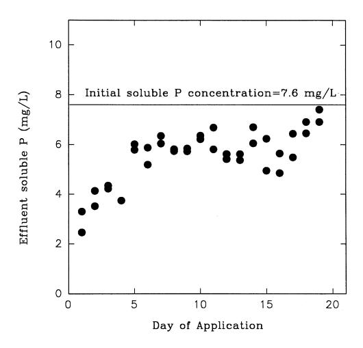
Figure 11. Removal of soluble P from alligator farm wastewater in land application system at  $1.0\ \mathrm{cm/day}$  loading rate.
