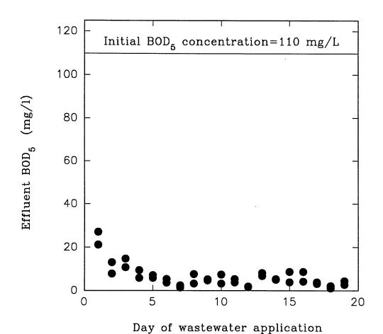
Figure 3. Removal of BOD from sugar refinery wastewater in land application system at 1.0 cm/day loading rate.
