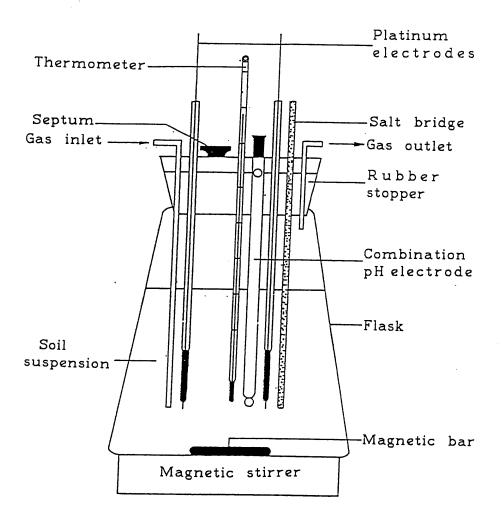
Figure 1. Controlled redox-pH microcosm.
