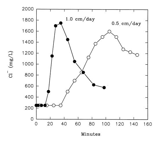
Figure 5. Detention time measurement using  ${\rm C1}^-$  as a conservative tracer for loading rates of 0.5 and 1.0 cm/day.
