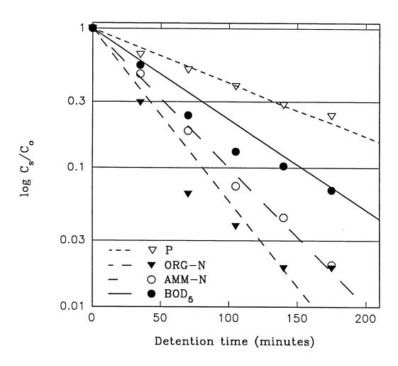
Figure 1. Summary of removal rate data for phosphorus (P), organic N (ORG-N), ammonia-N (AMM-N) and BOD (BOD $_5$ ) in land application system at a 1 cm/day loading rate.
