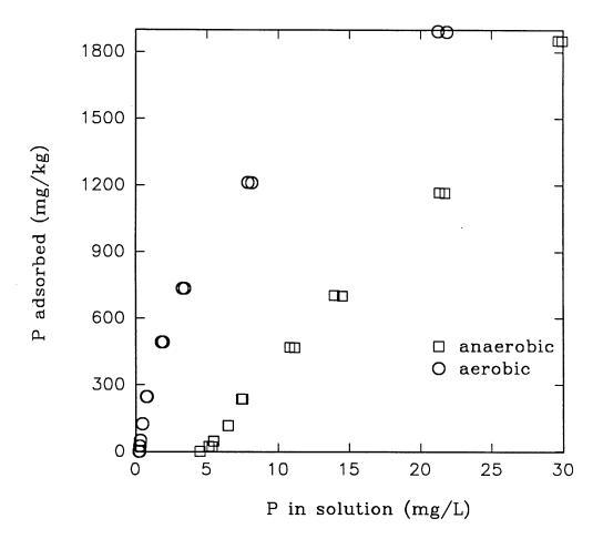
Figure 2. Adsorption isotherm for P under aerobic and anaerobic soil conditions.
