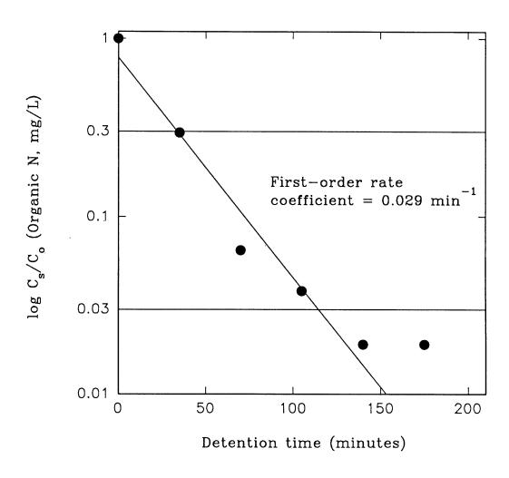
Figure 8. Removal of organic N during repeated application of alligator farm wastewater. Data are plotted as a first-order removal process. Experiment performed at 1.0 cm/day loading rate.
