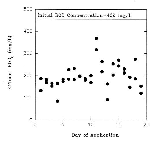
Figure 4. Removal of BOD from alligator farm wastewater in land application system at  $1.0\ \mathrm{cm/day}$  loading rate.
