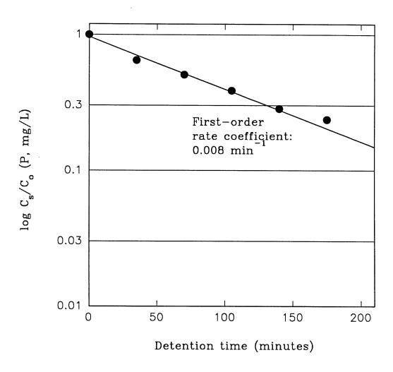
Figure 12. Removal of soluble P during repeated application of alligator farm wastewater. Data are plotted as a first-order removal process. Experiment performed at 1.0 cm/day laoding rate.
