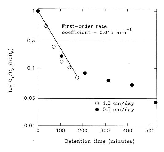
Figure 6. Removal of BOD during repeated application of alligator farm wastewater. Data are plotted as a first-order removal process. Experiments performed at two loading rates (0.5 cm/day and 1.0 cm/day).
