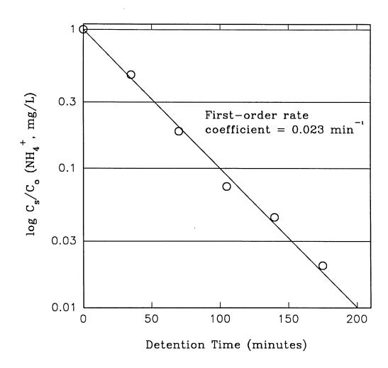
Figure 10. Removal of ammonia N during repeated application of alligator farm wastewater. Data are plotted as a first-order removal process. Experiment perfomed at 1.0 cm/day loading rate.
