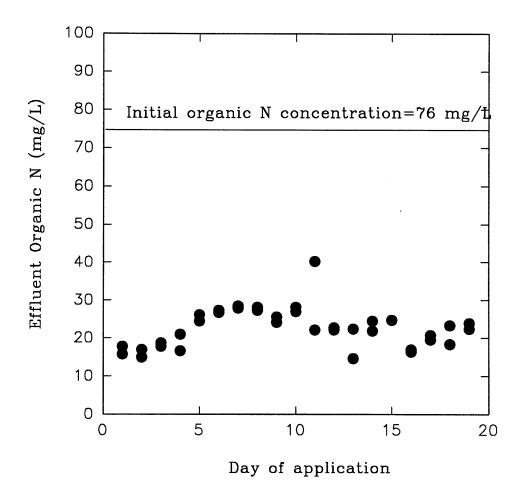
Figure 7. Removal of organic N from alligator farm wastewater in land application system at 1.0 cm/day loading rate.
