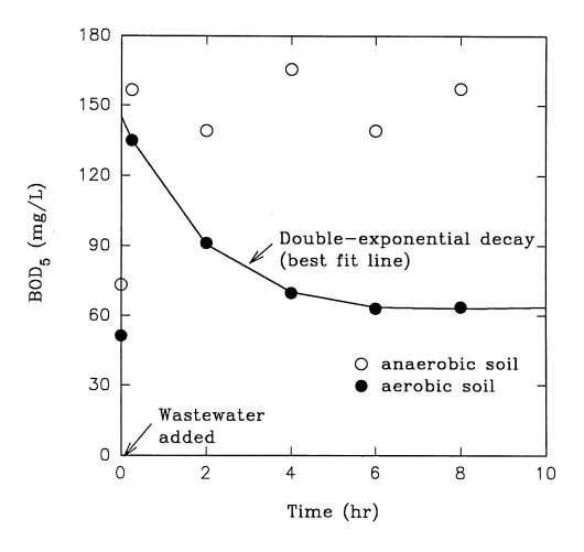
Figure 1. Decay of BOD in controlled microcosms under aerobic and anaerobic conditions. Solid line is from non-linear fit of double-exponential decay equation.
