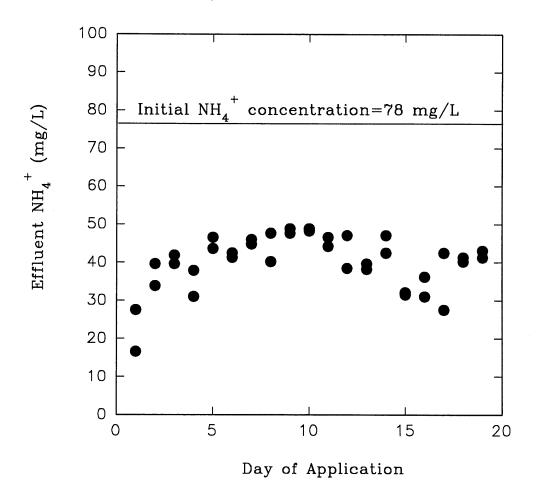
Figure 9. Removal of ammonia N from alligator farm wastewater in land application system at 1.0 cm/day loading rate.
